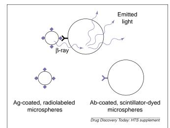
**Figure 1.** Scintillation proximity assays. If the antibody (Ab) reacts with the antigen (Ag) to bind these particles together, light will be released when β-rays emitted from antigen-coated microspheres enter the antibody-coated, scintillator-dyed microspheres. Free antigen in the sample will interfere with the binding of the two microspheres and will decrease light output.
